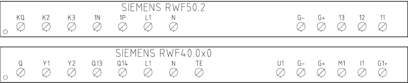
Matches terminals between RWF50.2 and RWF40.0x0
