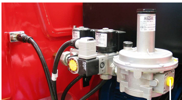
connection to the gas supply network - 1/2"
