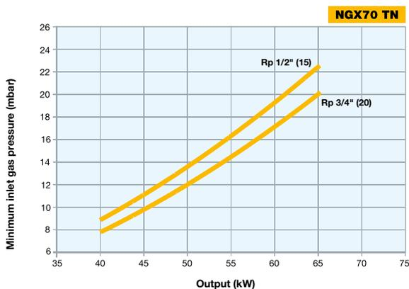
Attention: the graph shows the value of the gas output (kW) against the corresponding pressure without the combustion chamber back pressure. To know the minimum gas pressure at gas train, in order to get the gas output, it is necessary to add the boiler back pressure to the value read on the curve.
