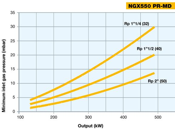
Attention: the graph shows the value of the gas output (kW) against the corresponding pressure without the combustion chamber back pressure. To know the minimum gas pressure at gas train, in order to get the gas output, it is necessary to add the boiler back pressure to the value read on the curve.
