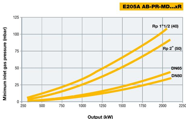
**Attention:** the graph shows the value of the gas output (kW) against the corresponding pressure without the combustion chamber back pressure. To know the minimum gas pressure at gas train, in order to get the gas output, it is necessary to add the boiler back pressure to the value read on the curve.
