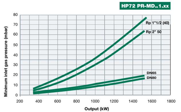
Attention: the graph shows the value of the gas output (kW) against the corresponding pressure without the combustion chamber back pressure. To know the minimum gas pressure at gas train, in order to get the gas output, it is necessary to add the boiler back pressure to the value read on the curve.
