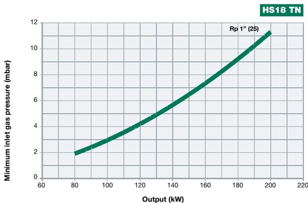
Attention: the graph shows the value of the gas output (kW) against the corresponding pressure without the combustion chamber back pressure. To know the minimum gas pressure at gas train, in order to get the gas output, it is necessary to add the boiler back pressure to the value read on the curve.
