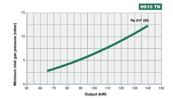
Attention: the graph shows the value of the gas output (kW) against the corresponding pressure without the combustion chamber back pressure. To know the minimum gas pressure at gas train, in order to get the gas output, it is necessary to add the boiler back pressure to the value read on the curve.
