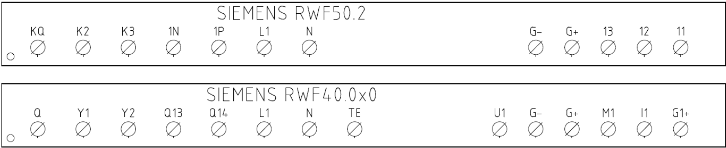
Matches terminals between RWF50.2 and RWF40.0x0
