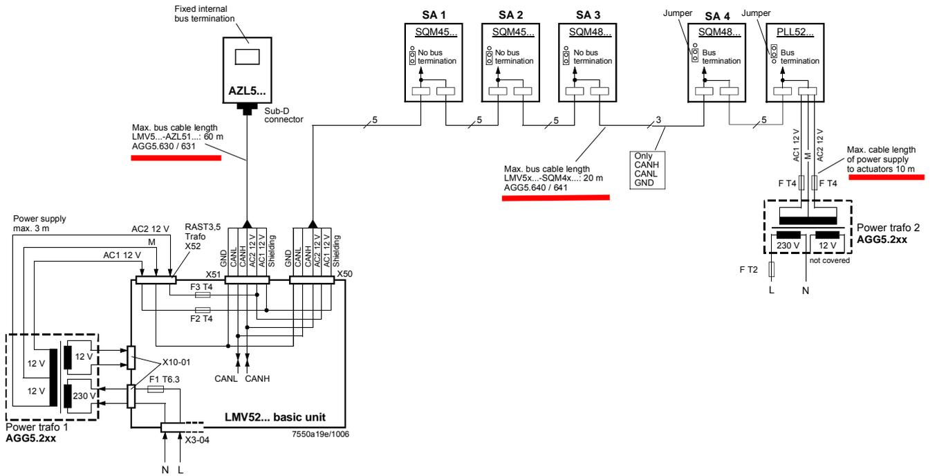
On LMV52... applications with more than 4 actuators (SQM45...), a second transformer is required for powering the extra actuators.
