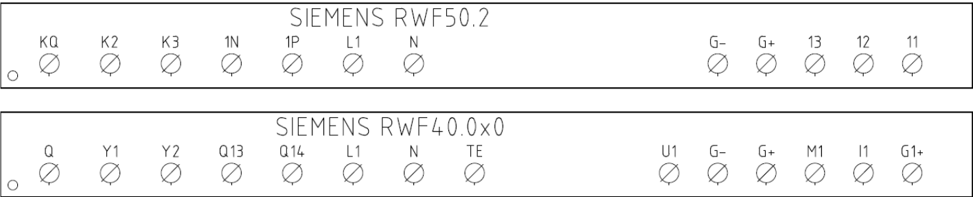
Matches terminals between RWF50.2 and RWF40.0x0
