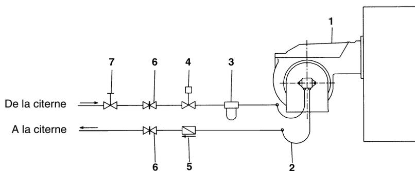
Fig. 6 - Installation bitube
