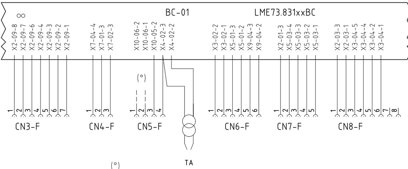
SONDA "UV" IN ALTERNATIVA A ELETTRODO "ER"
