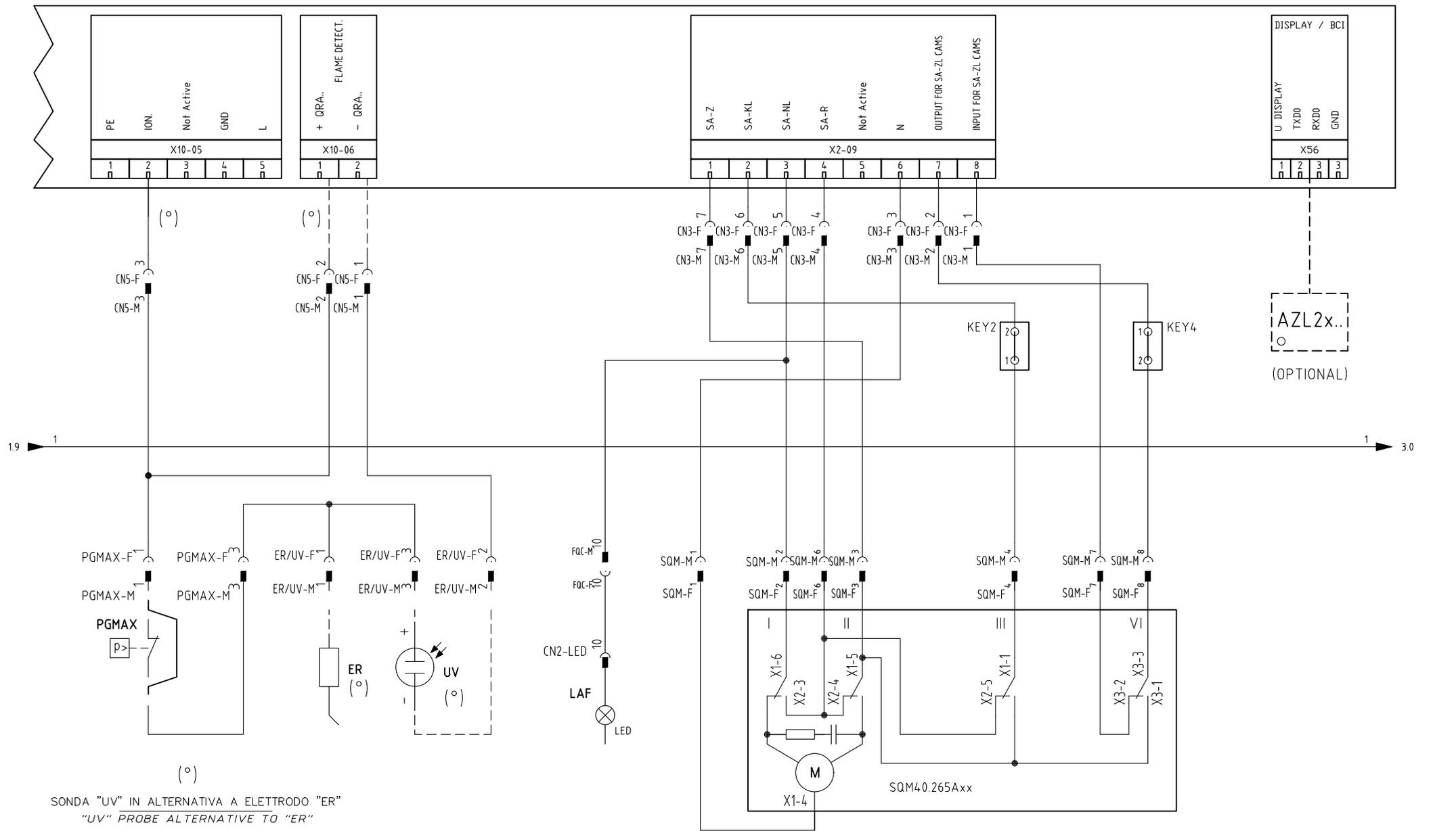
SONDA "UV" IN ALTERNATIVA A ELETTRODO "ER"
